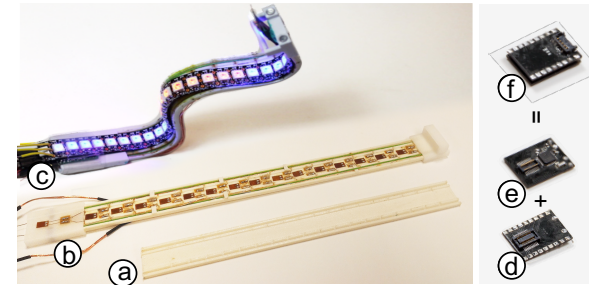
Figure 2: fStrip prototype. (a) NinjaFlex substrate, (b) fStrip with iron wires, (c) fStrip with 9DOF IMU and LED strip, (d) strain gauge breakout board, (e) main board (f) stacking main board and breakout board.
