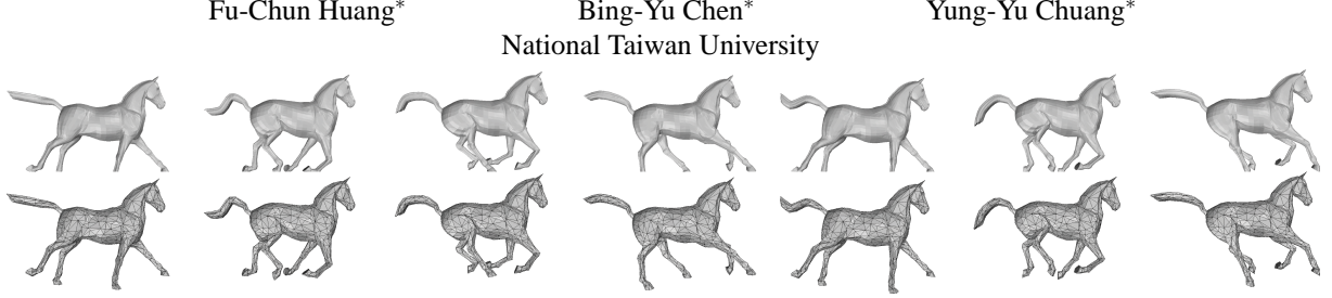
Figure 1: A horse-gallop animation with 48 frames. Upper: The original animation with 16,843 faces. Bottom: 1,588 faces approximation.
