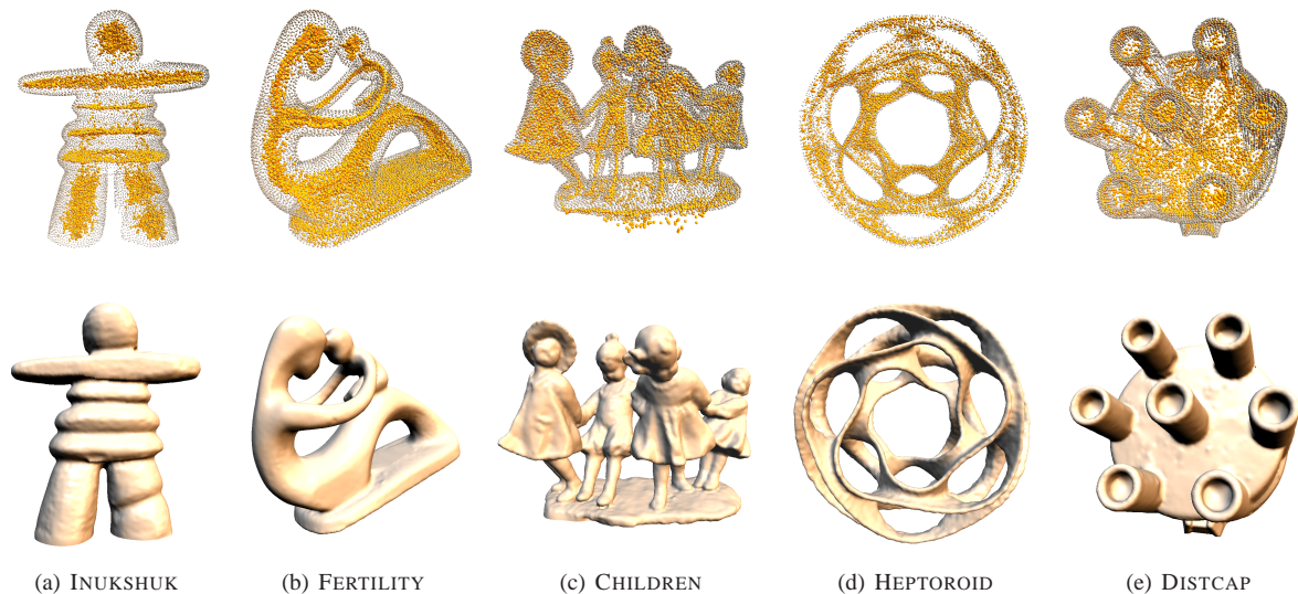
Figure 9: BPC assisted surface reconstruction. Top: The input point sets and their interior poles \mathcal{P}^- colored in coral. Bottom: The corresponding reconstructed RBF implicit surfaces.
