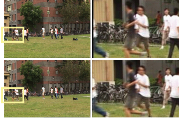
Figure 8: Upper-Left: The frame after aligning to the stabilized camcorder motion path. There is a missing area at the left side and a moving object across the missing area. Lower-Left: The result of dynamic region completion. Right Column: The close-up view of the yellow rectangles in the Left Column.
