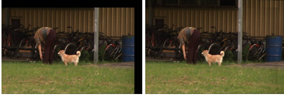
Figure 9: Left: The frame after changing the position according to the stabilized camcorder motion path. There is a missing area at the right side and upper side. Right: The result of static region completion. Since the missing area is large, there is a discontinuity boundary between the recovered pixels and the original frame.
