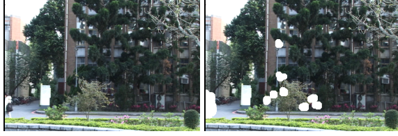
Figure 6: Left: The frame after aligning to the stabilized camcorder motion path. Right: The mask of detected moving objects (white regions).
