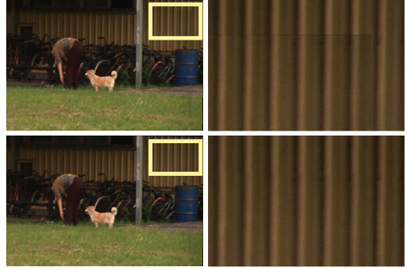
Figure 10: Upper-Left: The frame after video completion. Since the missing area is large, there is a discontinuous boundary between the recovered pixels and the original frame. Lower-Left: The result of video completion with Poisson-based smoothing. Right Column: The close-up view of the yellow rectangles in the Left Column.
