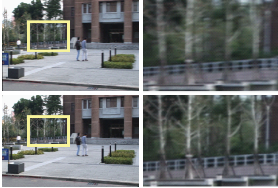
Figure 11: Upper-Left: A blurry frame. Lower-Left: The result of video deblurring. Right Column: The close-up view of the yellow rectangles in the Left Column.
