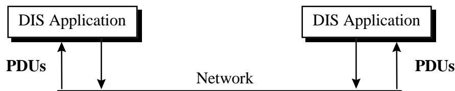
Figure 4-1 The control flow of DIS. A DIS application needs to maintain all the simulation information necessary, and uses PDUs to communicate with each other.
