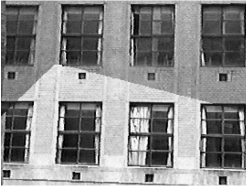
Photo.2 Part of the environment map generated by ordinary ray-casting. There is obvious intensity discontinuity.
