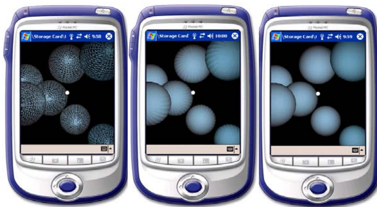
Figure 3. The results of three classic shading and lighting algorithms on a Pocket PC 2003 emulator.
