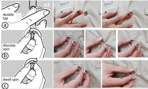
Figure 4. Three input methods are implemented: (a) tap input, (b) discrete spin, and (c) dwell spin
