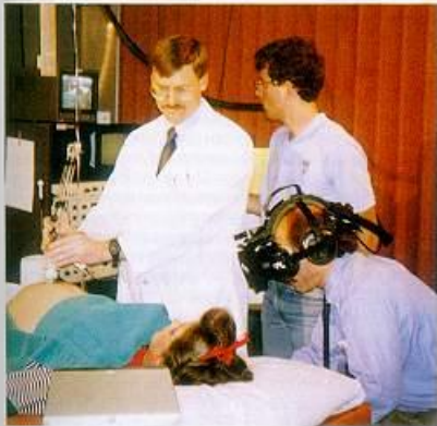
Figure 4. An ultrasound technician scans a subject while another person looks on with the video see-through head-mounted display (HMD). Note the miniature video camera attached to the front of the VPL EyePhone HMD.
